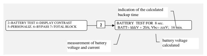
This activates the cycle to check the state of efficiency of the battery, which lasts 8 seconds. Press key 8 to interrupt the test and return to the basic menu before this time has elapsed.
