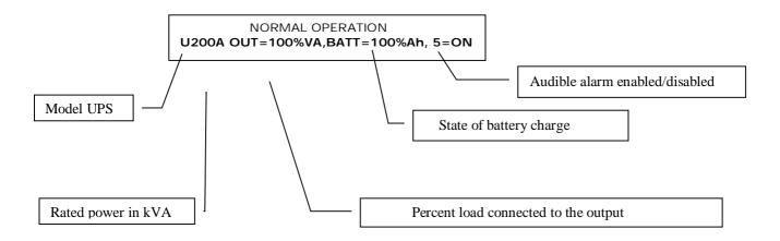
The message U200A indicates an UPS model with 200kVA rated power, operating with 60Hz output frequency. When the unit is set for the parallel operation the letter "P" is added (U200AP). The letter "P" became lower case "p" when the unit operate as slave.
