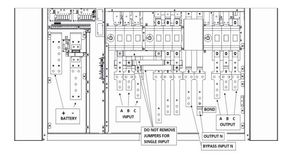
MASTER HP - UL 400 kVA and 500 kVA with TCE Power connection Terminals
