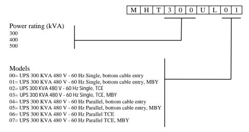
e.g .: MHT 300 UL-01; UPS 300kVA single unit, bottom cable entry and switch maintenance bypass present.
