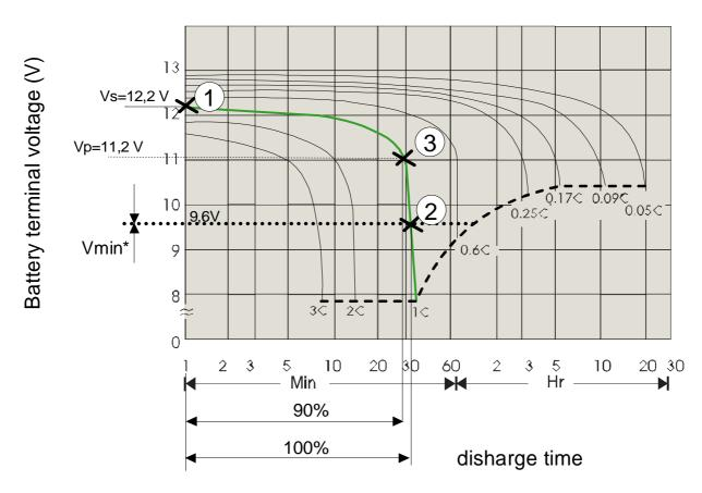
The three values, Vs, Vmin and Vp, are obtained from the discharge characteristic curve, supplied from manufacturer, relating to the *battery discharge regime* 1C has been determined:
