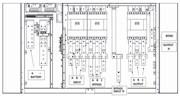
Remove the jumpers present between the BYPASS and INPUT bars.
