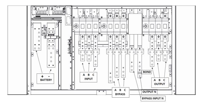
MASTER HP - UL 400 kVA and 500 kVA TCE Power connection Terminals
