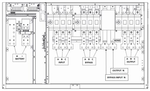
MASTER HP - UL 400 kVA and 500 kVA Power connection Terminals
