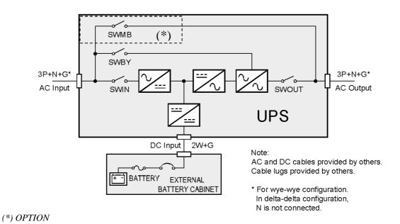
Schematic diagram: Dual input Unit
