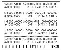
This key switch to page with all codes and measurements displayed of 1 event. The key "6" switch from code with message line to full lines code.
