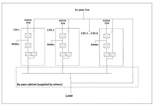
Note: For parallel system greater than 1+1 redundant, it's recommended to install the wrap around bypass switch. This is to assure the correct maintenance.
