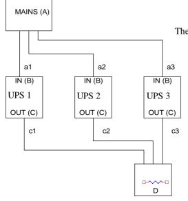
The figure shows an example of three units connected in parallel.
