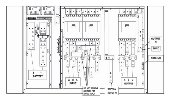
Note: When cables entering from the top, respect the following order: connecting cables to the Input terminals first and Battery terminals then, and in the same way, connecting cables to the Bypass terminals first and Output terminals then. The label marked "N" present on the terminal identifies the neutral terminal. Maintenance Bypass Switch optional.
