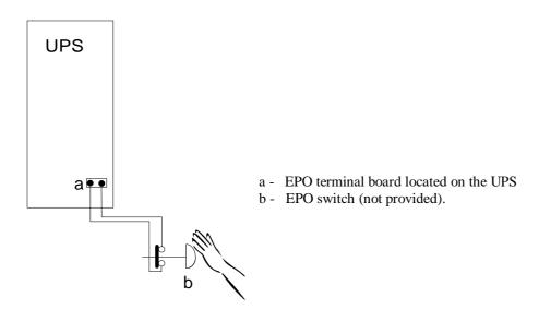
On the UPS, the jumper on the EPO terminals must be removed, and the wires from the auxiliary contact of the button must be connected in place of the jumper.
