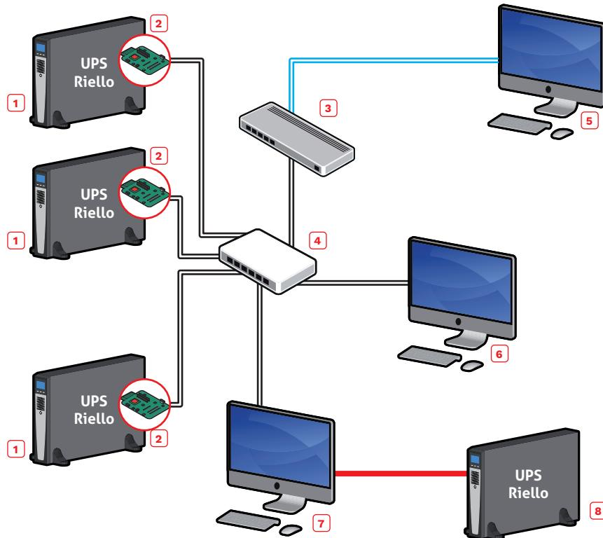
Connection with more than 1 UPS. The FULL version of PowerShield<sup>3</sup> software is required as well as a NetMan 208C communication board on each UPS.
