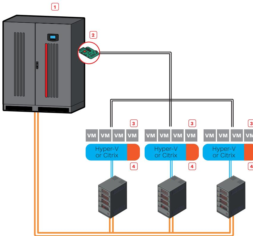
PowerShield<sup>3</sup> software should be used for managing setup with UPS, a specific script to shut down the virtualised system must be used, UPS must have a NetMan 208C board installed.
