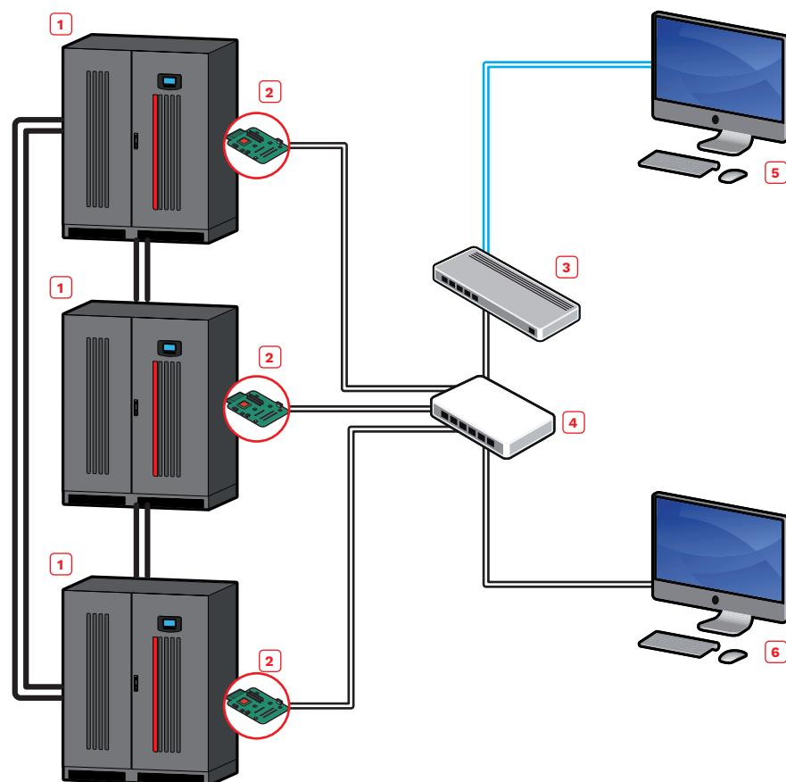
The FULL version of PowerShield<sup>3</sup> software should be used for managing setups with several UPS installed in parallel and each UPS must have a NetMan 208C board installed.
