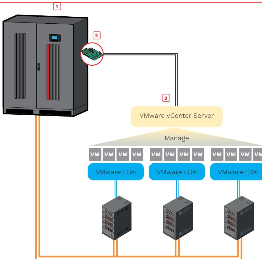
NetMan 208C should be used for managing Esxi hosts and vCenter servers, enabling you to manage your virtual network to perform shutdown or live migrations of active virtual machines as well as shutdown of physical hosts with delay and priority.
