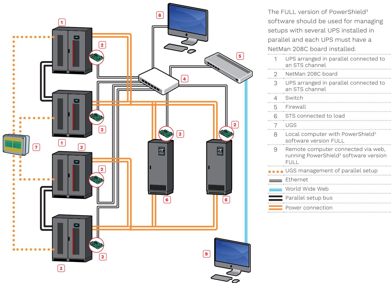
The FULL version of PowerShield<sup>3</sup> software should be used for managing setups with several UPS installed in parallel and each UPS must have a NetMan 208C board installed.
